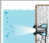
Water must be allowed to go inside and outside sleeve freely without leaking to the other side.
